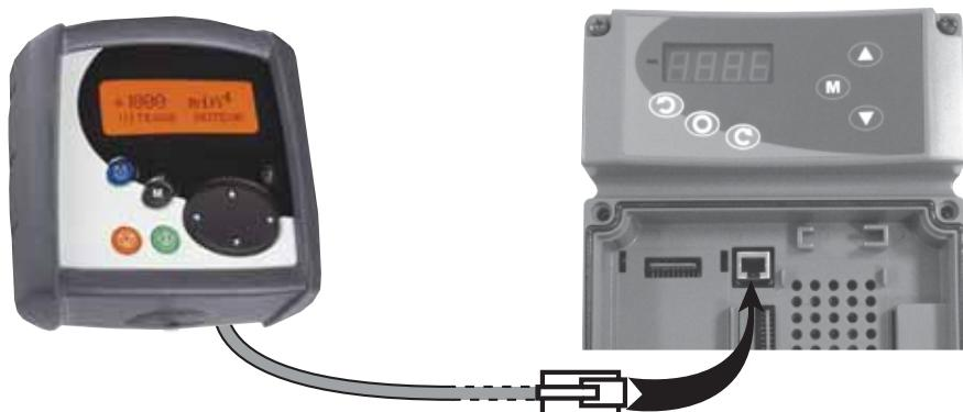
The drive automatically detects the presence of the LCD keypad.
